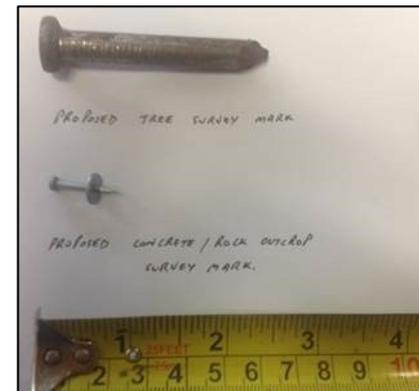
Survey monitoring 'pins' for subsidence monitoring 11
